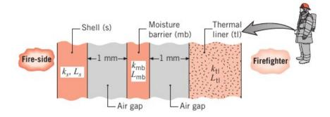
Representative dimensions and thermal conductivities for the layers are as follows.
