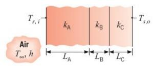
Under steady-state operating conditions, measurements reveal an outer surface temperature of  $T_{s,o} = 20^{\circ}\text{C}$ , an inner surface temperature of  $T_{s,i} = 600^{\circ}\text{C}$ , and an oven air temperature of  $T_{\infty} = 800^{\circ}\text{C}$ . The inside convection coefficient h is known to be 25 W/m<sup>2</sup>·K. What is the value of  $k_{\rm B}$ ?
