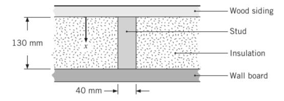
What is the thermal resistance associated with a wall that is 2.5 m high by 6.5 m wide (having 10 studs, each 2.5 m high)? Assume surfaces normal to the *x*-direction are isothermal.
